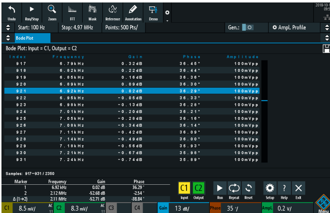
A table of measurement results provides detailed information about each measurement point, consisting of frequency, gain and phase shift
