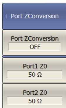
This function converts the S-parameters measured at a 50 or 75 Ω port into values which would be seen if measured at a test port with arbitrary impedance.
