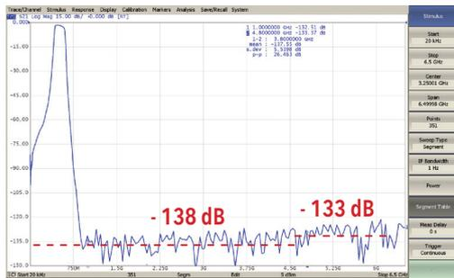
Typical dynamic range of 125 dB is achieved from 300 kHz through the top of the frequency range (at 10 Hz IF bandwidth). Seen here is the maximum dynamic range achieved when using IFBW 1 Hz and an output power level of 5 dBm.
