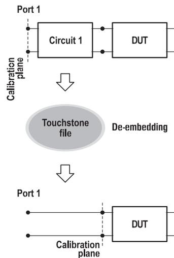
Allows users to mathematically exclude from the measurement result the effect of the fixture circuit connected between the calibration plane and a DUT. This circuit should be described by an S-parameter matrix in a Touchstone file.
