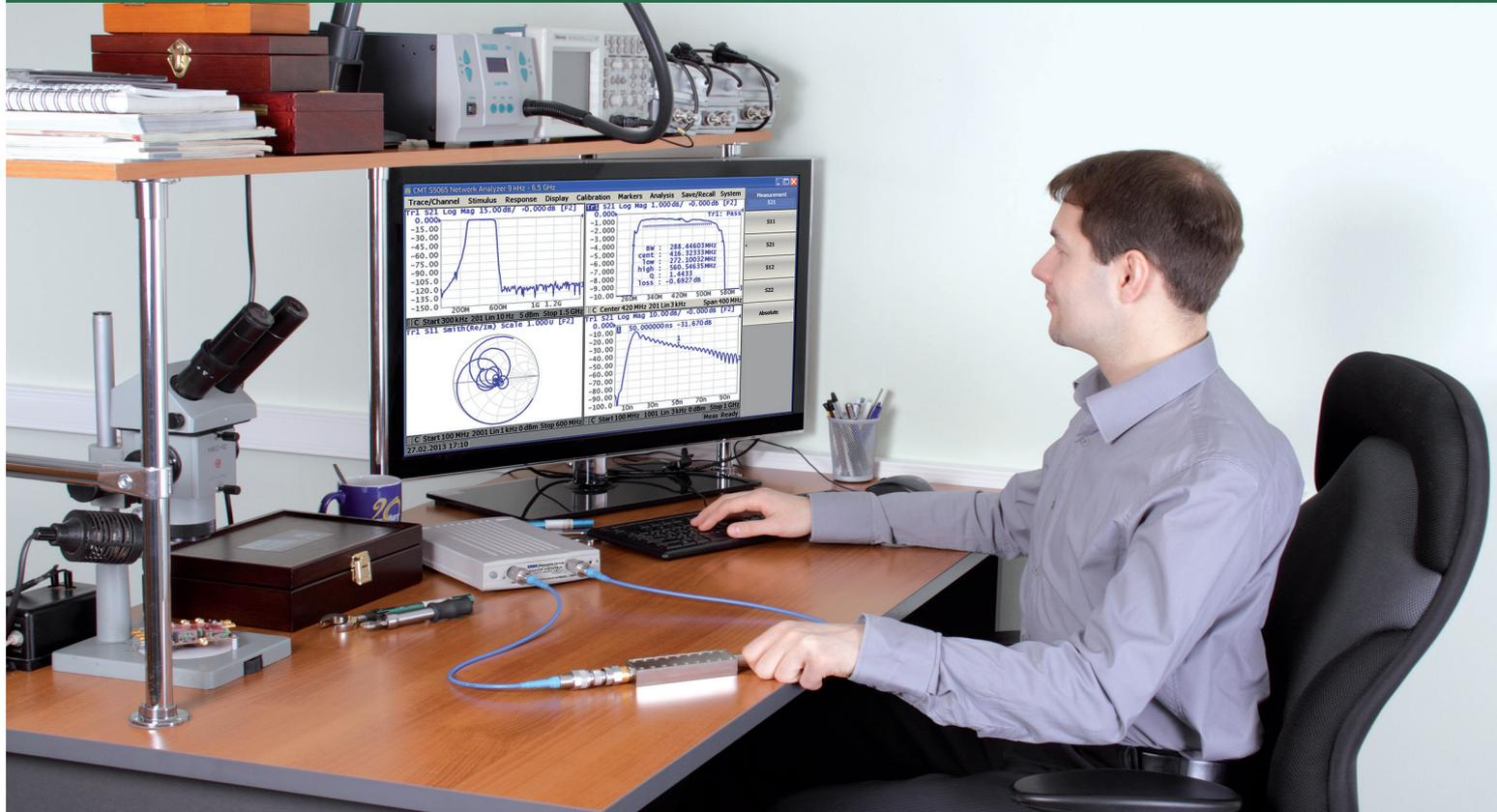
Our Compact Series VNAs deliver lab grade performance in a compact package, with all the features engineers have come to expect included: time domain and gating conversion, segmented frequency sweeps, linear/logarithmic sweeps, power sweeps, multiple trace formats, 16 channels max. with up to 16 traces each, marker math, and limit tests.
