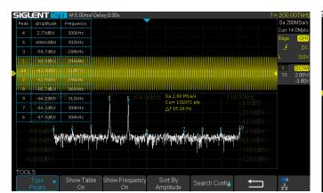
The new math co-processor enables FFT analysis of incoming signals using up to 128k samples per waveform. This provides high frequency resolution with a fast refresh rate. The FFT function also supports a variety of window functions so that it can adapt to different spectrum measurement needs. Four-channel series support Peaks, Markers, a variety of numbers.
