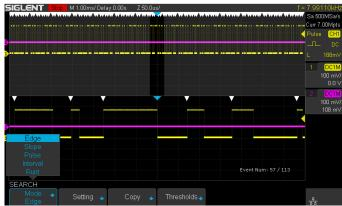
The SDS1000X-U can search events specified by the user in a frame. It can also navigate by time (delay position) and historical frames.
