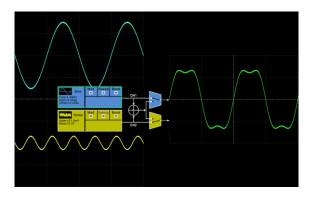
Waveform Combining Superimposes CH1 and CH2 waveforms internally and provides the combined waveform to a user-selected output. It easily combines basic waveforms, random noise, modulation signals, sweep signals, burst signals, EasyPulse waveforms, and TrueArb waveforms without external connections or complex editing.
