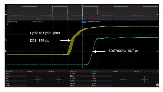
**Low jitter** When a Square/Pulse waveform is generated by traditional DDS, there can be additional jitter if the sample rate is not an integer-related multiple of the output frequency. EasyPulse technology successfully overcomes this weakness in DDS designs and helps to produce low jitter Square/Pulse waveforms.
