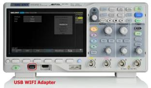
WiFi control of instrumentation can provide a convenient and safe method of configuring and collecting data. This new feature works with a SIGLENT approved WiFi adapter to provide wireless control and communications with SIGLENT 4 channel scopes. The adapter must be supplied by Siglent to ensure working. USB 25 MHz AWG Module (four channel series only, option)
