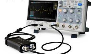
The four channel series supports a USB 25 MHz function/arbitrary waveform generator that is operated from the USB host connection. Functions include Sine, Square, Ramp, Pulse, Noise, DC and 45 built-in waveforms. The arbitrary waveforms can be accessed and edited by the SIGLENT EasyWave PC software.
