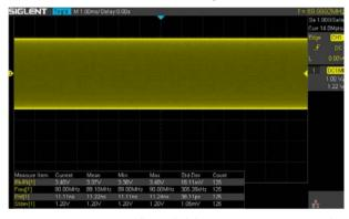
SDS1004X-E can measure all sampled data points up to 14 Mpts. This ensures the accuracy of measurements while the math co-processor decreases measurement time and increases ease-of-use.
