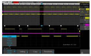
The SDS1000X-E can search events specified by the user in a frame. It can also navigate by time (delay position) and historical frames.
