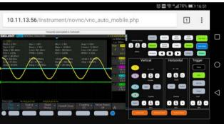
With the new embedded web server, users can control the SDS1xx4X-E from a simple web page. This provides wonderful remote troubleshooting and monitoring capabilities. The web page has PC and mobile styles that include an embedded virtual control panel
