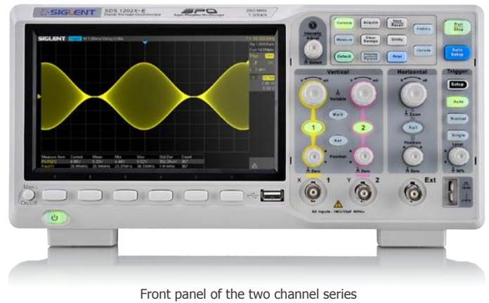
Front panel of the two channel series
