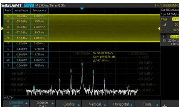
The new math co-processor enables FFT analysis of incoming signals using up to 1 M samples per waveform. This provides high frequency resolution with a fast refresh rate. The FFT function also supports a variety of window functions so that it can adapt to different spectrum measurement needs. Four-channel series support Peaks, Markers, a variety of numbers.
