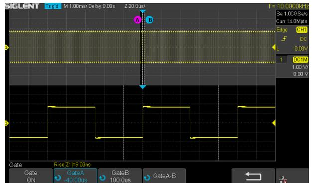
Through Gate and Zoom measurement, the user can specify an arbitrary interval of waveform data analysis and statistics. This helps avoid measurement errors that can be caused by invalid or extraneous data, greatly enhancing the measurements' validity and flexibility.
