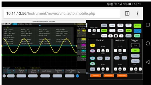
With the new embedded web server, users can control the SDS1xx4X-E from a simple web page. This provides wonderful remote troubleshooting and monitoring capabilities. The web page has PC and mobile styles that include an embedded virtual control panel
