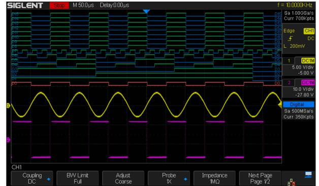
16 digital channels enables users to acquire and trigger on the waveforms then analyze the pattern, simultaneously with one instrument.
