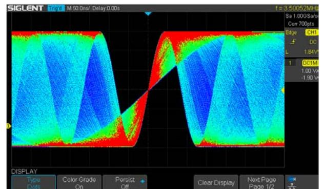
The color temperature display is similar to the intensity-graded trace function, but the trace occurrence is represented by different colors (color "temperature") as opposed to changes in the intensity of one color. Red colors represents the more frequent events, while blue is used to mark points that occur least frequently.
