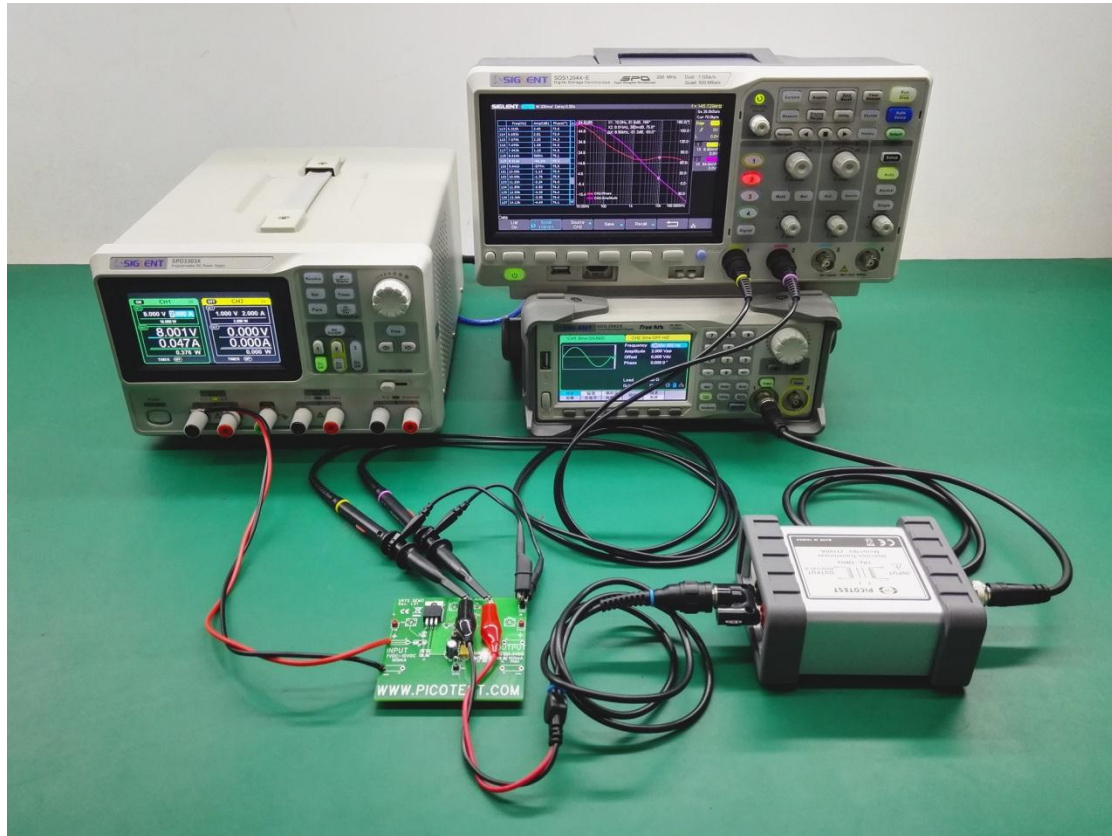
Figure 1 Set Up for the Bode Plot Measurement
