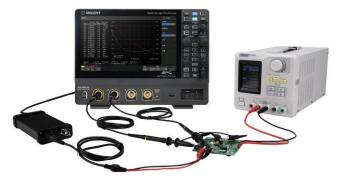
SDS1000X HD can control the USB AWG module or control an independent SIGLENT SDG instrument, scan a devices amplitude and phase frequency response, and display the data as a Bode Plot. There is also a Vari-level Mode for accurately measuring Power Supply Control Loop Response (PSRR).
