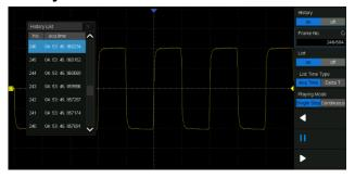
History function can record up to 80,000 frames of waveforms. The recording is executed automatically so that the customer can playback the history waveforms at any time to observe unusual events and quickly locate the area of interest using the cursors or measurements.
