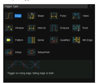
Edge, Slope, Pulse width, Video, Windows, Runt, Interval, Dropout, Pattern, Qualified, Nth edge, Delay, Setup/Hold time, and serial trigger.
