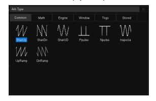
The USB waveform generator can output waveforms with up to 25 MHz frequency and ±3 V amplitude. Six basic waveforms together with multiple types of predefined waveforms and as user-defined arbitrary waveforms are supported.
