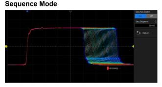
Segmented memory collection will store the waveform into multiple memory segments (up to 80,000) and each segment will store a triggered waveform as well the dead time information. The interval between segments can be as small as 2  $\mu$ s. All of the segments can be played back using the History function.
