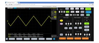
With the new embedded web server, users can control the SDS2000X-E from a simple web page. This provides wonderful remote troubleshooting and monitoring capabilities. The web page has PC and mobile styles that include an embedded virtual control panel.
