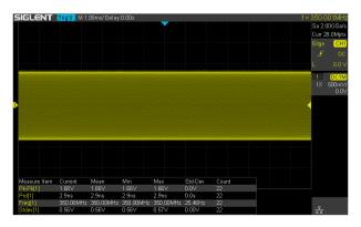
SDS2000X-E can apply automatic measurements on all sampled data points up to 28 Mpts. This ensures the accuracy of measurements while the math co-processor decreases measurement time and increases ease-of-use.
