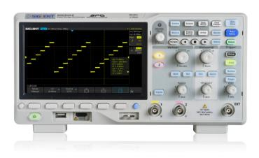
• 7-inch TFT-LCD display with 800 \* 480 resolution
