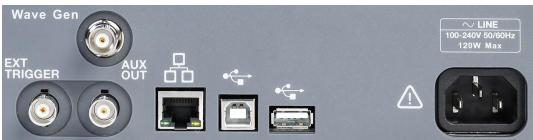
USB Host 2.0 x3, USB Device 2.0 (USBTMC) , LAN (VXI-11/Telnet/Socket), Auxiliary output (Pass/Fail, Trigger Out), etc.
