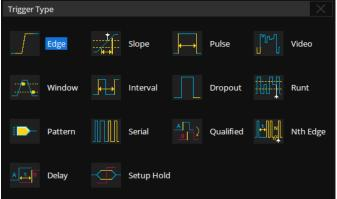
Edge, Slope, Pulse, Video, Windows, Runt, Interval, Dropout, Pattern, Qualified, Nth edge, Setup/hold, Delay, and serial trigger
