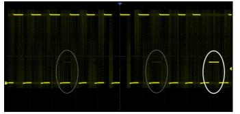
With a waveform update rate of up to 100,000 wfm/s, the oscilloscope can easily capture unusual or low-probability events. In Sequence mode, the waveform capture rate can reach 500,000 wfm/s
