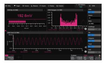
4-digit voltmeter and 7-digit frequency counter. Any analog channel can be selected as a source. Bar, Histogram and Trend diagrams are supported
