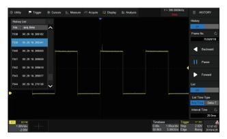
History function can record up to 100,000 frames of waveforms. The recording is executed automatically, so that the customer can play back the history waveforms at any time in order to observe unusual events and quickly locate the area of interest using the cursors or measurements
