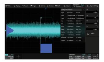
The Waveform Histogram feature provides a statistics view of the waveform in horizontal and vertical directions
