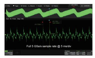
Using hardware-based Zoom technique and record length of up to 250 Mpts, users can select a slower timebase without compromising the sample rate, and then quickly zoom in to focus on the area of interest
