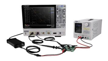
The oscilloscope can control the isolated USB AWG module or a stand-alone SIGLENT SDG generator, to scan the amplitude and phase-frequency response of the DUT, and display the data as a Bode Plot. This makes it possible to replace expensive network analyzers in some applications
