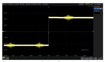
Segmented memory collection will store the waveform into multiple memory segments (up to 124,000) and each segment will store a triggered waveform as well the dead time information. The interval between segments can be as small as 0.9  $\mu s$ . All of the segments can be played back using the History function
