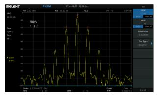
Phase noise -98 dBc/Hz@ 1 GHz, offset 10 kHz
