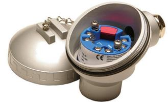
100 ohm Pt RTD or 0-900 ohm input ◆ 4-20mA output ◆ Loop-powered, 9-32V DC
