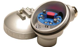
Thermocouple (8 types) or ±100mV input ♦ 4-20mA output ♦ 1500V isolation ♦ Loop-powered
