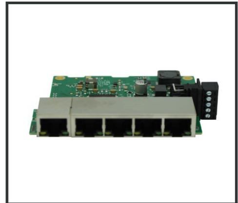
Embedded format, takes up minimal space, with mounting holes connected to Functional Earth
