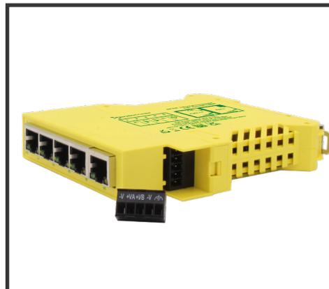
Non conducting polyamide casing with removable numbered power terminal for easy wiring
