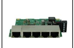
Embedded format, takes up minimal space, with mounting holes connected to Functional Earth
