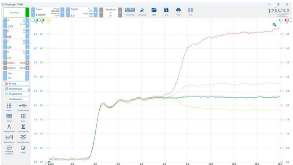
Screenshot: The effect of correct termination for “electrically long” signals
