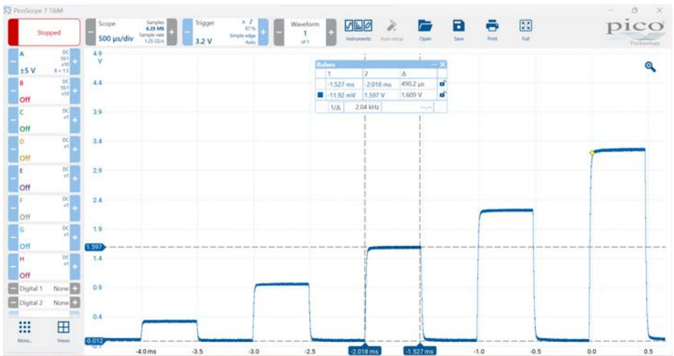
Screenshot: Measuring a pulse with the cursor function
