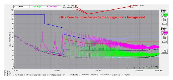
Charts are always saved including the amplitude correction data. If you figure out, that you applied wrong correction files, after completing a measurement, you can save the chart and then reload it as raw data and select different amplitude correction files.
