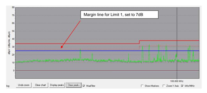
By default, the margins are set to 0, so any peak crossing the limit line would be indicated. Setting margin1 to e.g. 7dB would select all peaks coming within 7 dB close to the limit line of the graph measured with Settings1. Peaks crossing the margin line or limit line can be listed in the in the **Peaks window** by pressing the **Display peaks** button.
