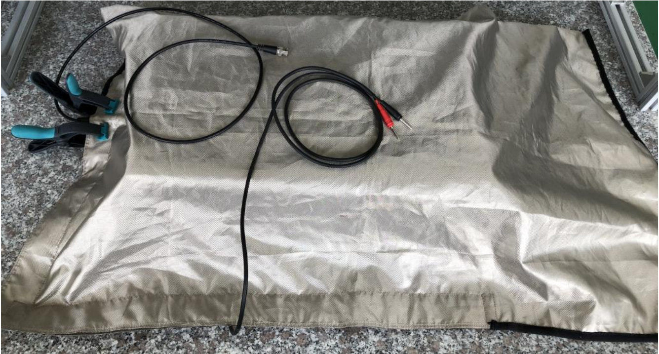
Picture 8: TBSB-105/60, conducted noise measurement set up inside
