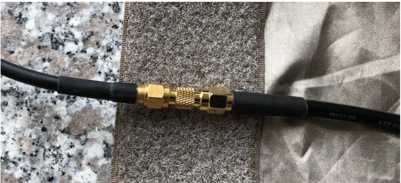
Picture 9: feed through using coaxial adapter
