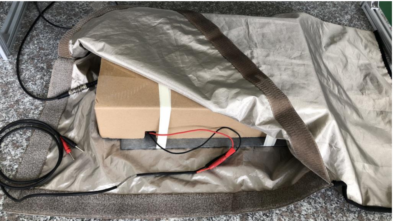
Picture 7: TBSB-105/60, preparing conducted noise measurement set up
