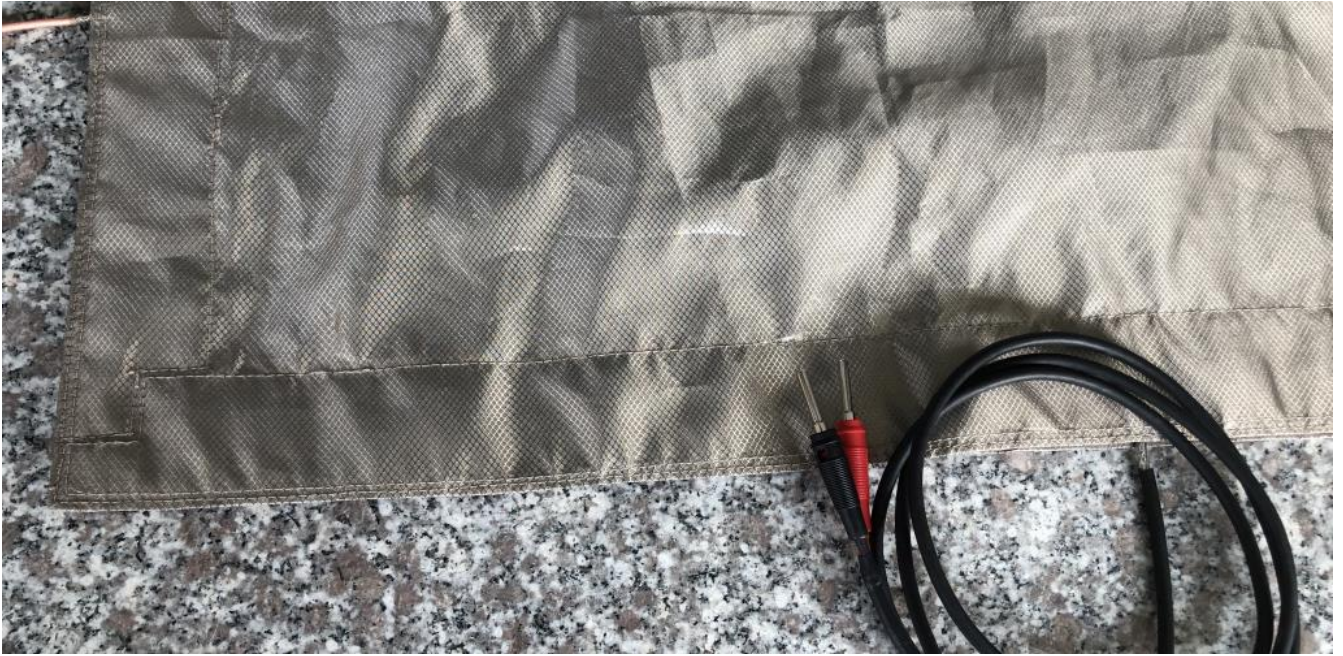
Picture 15: DUT supply feed through using a shielded cable with stripped jacket; bag closed
