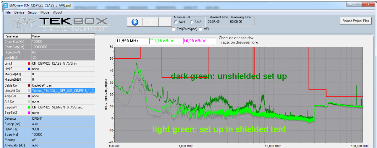
Picture 6: CISPR 25 conducted noise measurement; DUT powered
