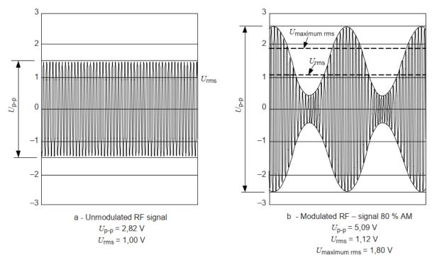
Consequently, the level of the modulated signal must be 5.1 dB higher than the test levels specified by the standard. Adding a 6dB attenuator to improve matching of the RF power amplifiers would require following amplifier output power:
