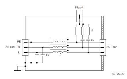
CDN-M3,  $C_1$  (typical) = 10 nF,  $C_2$  (typical) = 47 nF,  $R = 300 \Omega$ ,  $L \ge 280 \mu$ H at 150 kHz CDN-M2,  $C_1$  (typical) = 10 nF,  $C_2$  (typical) = 47 nF,  $R = 200 \Omega$ ,  $L \ge 280 \mu$ H at 150 kHz CDN-M1,  $C_1$  (typical) = 22 nF,  $C_2$  (typical) = 47 nF,  $R = 100 \Omega$ ,  $L \ge 280 \mu$ H at 150 kHz
