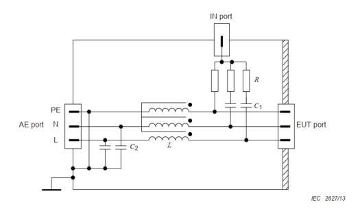
CDN-M3,  $C_1$  (typical) = 10 nF,  $C_2$  (typical) = 47 nF,  $R = 300 \Omega$ ,  $L \ge 280 \mu$ H at 150 kHz CDN-M2,  $C_1$  (typical) = 10 nF,  $C_2$  (typical) = 47 nF,  $R = 200 \Omega$ ,  $L \ge 280 \mu$ H at 150 kHz CDN-M1,  $C_1$  (typical) = 22 nF,  $C_2$  (typical) = 47 nF,  $R = 100 \Omega$ ,  $L \ge 280 \mu$ H at 150 kHz
