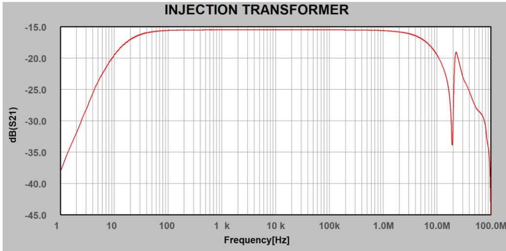
Figure 1: typical insertion loss
