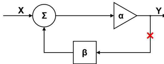
The isolation transformer is inserted into the control loop and connected to the Bode-Analyzer:
