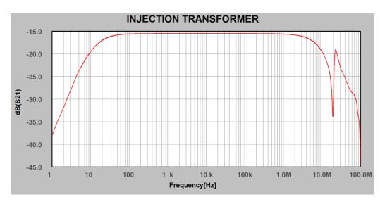
Figure 1: typical insertion loss
