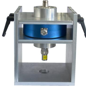
Picture 1: TBPCP4-CAL RF current probe calibration fixture
