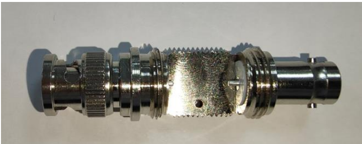
Picture 1: TBRFH7 RF housing components
