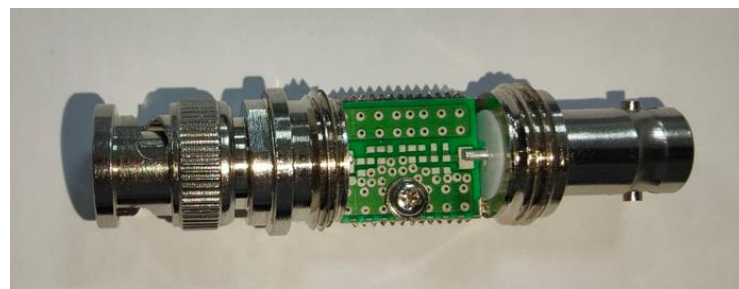
Picture 3: TBRFH7 RF housing application example – RF filter
