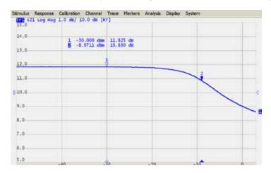
The power sweep feature turns compression point recognition, one of the most fundamental and complex amplified measurements, into a simple and accurate operation.
