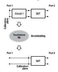
Allows users to mathematically exclude from the measurement result the effect of the fixture circuit connected between the calibration plane and a DUT. This circuit should be described by an S-parameter matrix in a Touchstone file.
