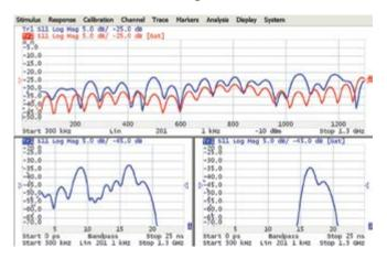
This function mathematically removes unwanted responses in the time domain, which allows the user to obtain a frequency response without effects of fixture elements.
