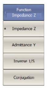
This function allows for conversion of measured S-parameters to the following parameters: reflection impedance and admittance, transmission impedance and admittance, and inverse S-parameters.
