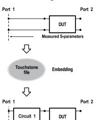
Allows the user to mathematically simulate the DUT parameters after virtual connection through a fixture circuit between the calibration plane and the DUT. This circuit is described by an S-parameter matrix in a Touchstone file.
