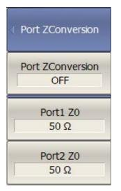
This function converts the S-parameters measured at a 50  $\Omega$  port into values which would be seen if measured at a test port with arbitrary impedance.
