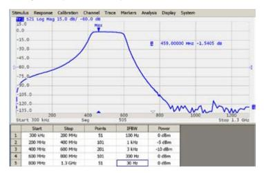
The VNA has a large frequency range with the option of frequency scan segmentation. This allows for optimal use of the device to realize the maximum dynamic range while maintaining high measurement speed.
