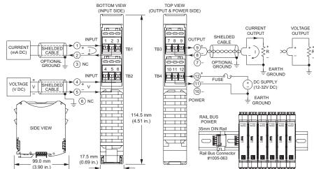
Multi-range ±20mA or ±500mV input ◆ Universal current/voltage output ◆ 12-32V DC local/bus power
