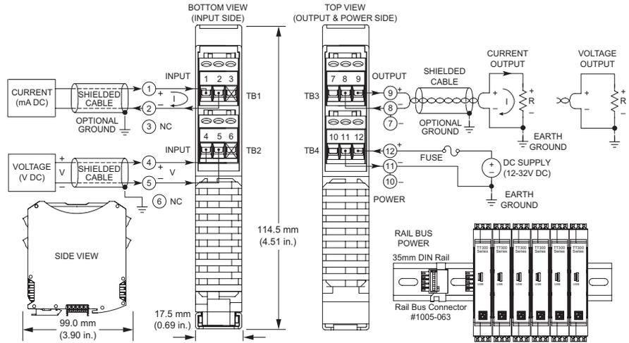
Multi-range  $\pm 20\text{mA}$  or  $\pm 500\text{mV}$  input ◆ Universal current/voltage output ◆ 12-32V DC local/bus power
