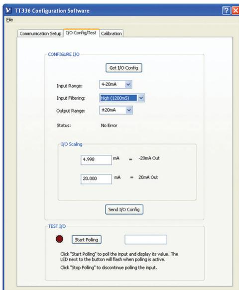
TT330 Series Transmitter Configuration Software is downloadable (FREE) from [www.acromag.com](http://www.acromag.com). Windows® XP, Vista, 7, and 8
