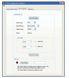
TT337 Model software allows you to configure transmitters offline, save the file, and download into units later, at your convenience.
