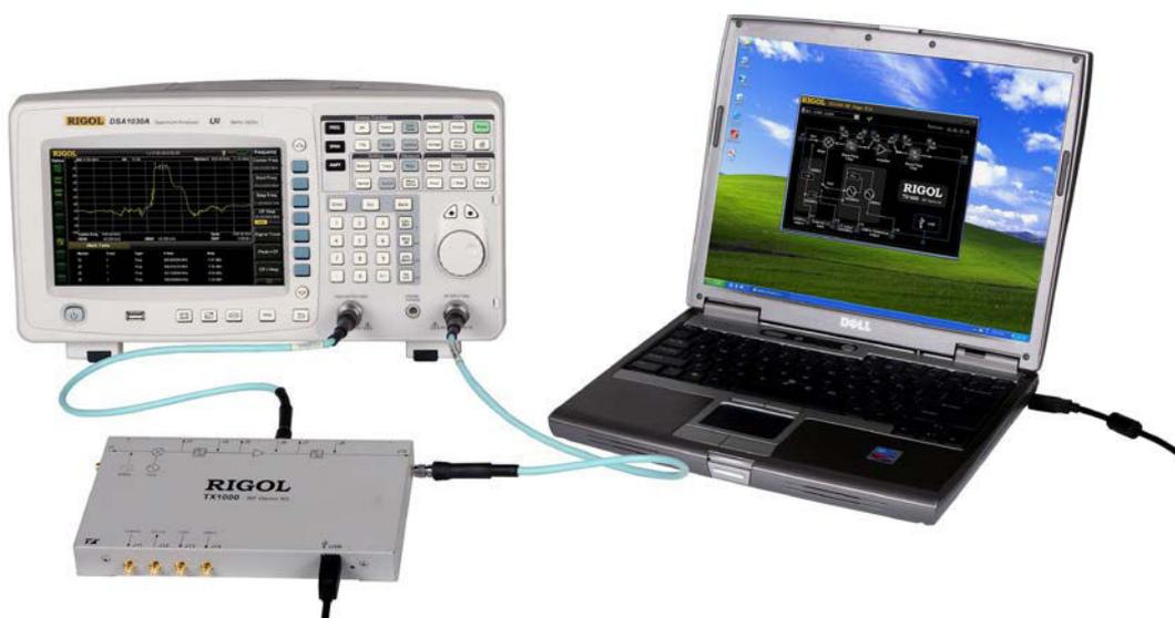
Figure 7 Test the Band-pass Filter Characteristics
