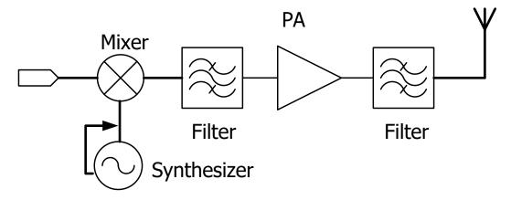
Figure 2 TX1000 Schematic Diagram
