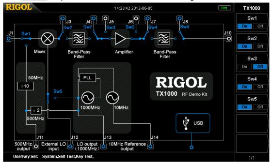
Figure 5 Built-in TX1000 Control Interface of DSA800
