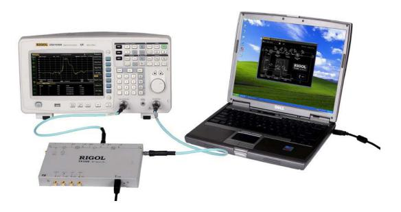
Figure 7 Test the Band-pass Filter Characteristics
