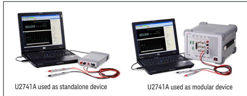
Figure 1. The U2741A DMM showing dual-play capability
