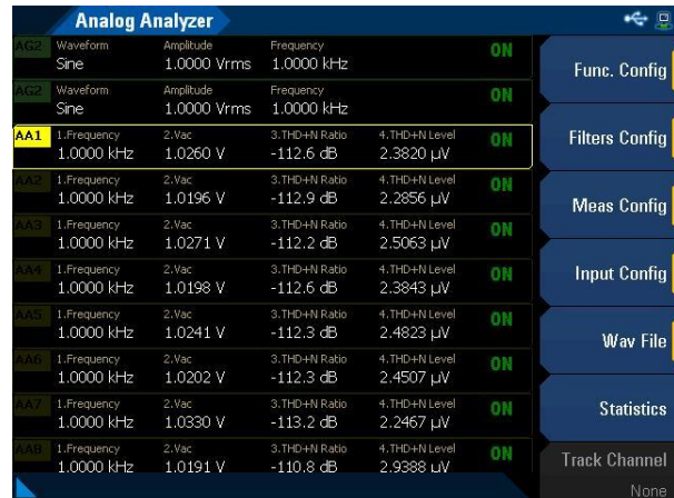
Figure 5. The U8903B's GUI, showing 8 analyzer channel measurements.
