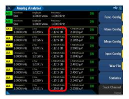
U8903B's GUI, showing 8 analyzer channel measurements
