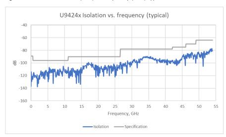
Figure 8. U9424x isolation vs frequency (GHz) typical
