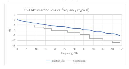
Figure 5. U9424x insertion loss vs frequency (GHz) typical
