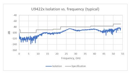
Figure 4. U9422x isolation vs frequency (GHz) typical
