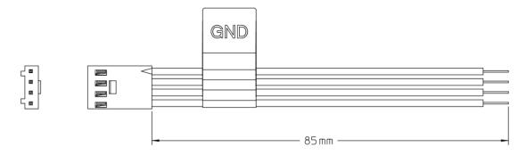
Figure 13. Option 101, 4-pins connector to bare wire, 85 mm (for SP4T option 001 only) dimension
