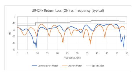
Figure 6. U9424x return loss (ON) vs frequency (GHz) typical
