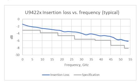
Figure 1. U9422x insertion loss vs frequency (GHz) typical
