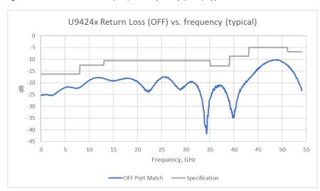
Figure 7. U9424x return loss (OFF) vs frequency (GHz) typical
