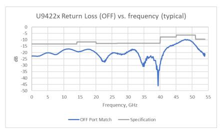
Figure 3. U9422x return loss (OFF) vs frequency (GHz) typical
