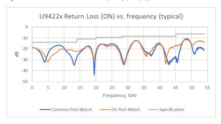
Figure 2. U9422x return loss (ON) vs frequency (GHz) typical
