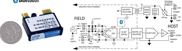
Bluetooth® wireless configuration option ◆ Narrow or wide band mV field input ◆ Voltage host output
