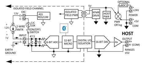
Bluetooth® wireless configuration option ◆ Narrow band DC current field input ◆ Voltage host output
