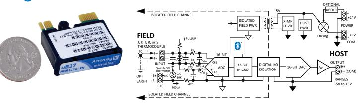
Bluetooth<sup>®</sup> wireless configuration option < Thermocouple field input < Voltage host output
