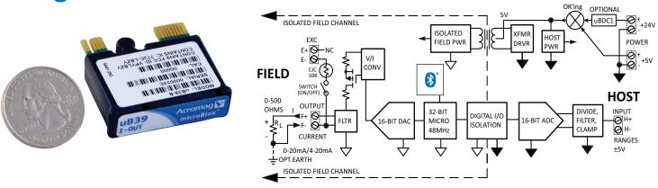
Bluetooth<sup>®</sup> wireless configuration option < DC current field output < Voltage host input
