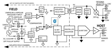
Bluetooth® wireless configuration option ◆ Frequency field input ◆ Voltage host output
