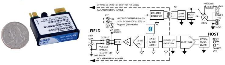
Bluetooth<sup>®</sup> wireless configuration option < DC voltage field output < Voltage field input
