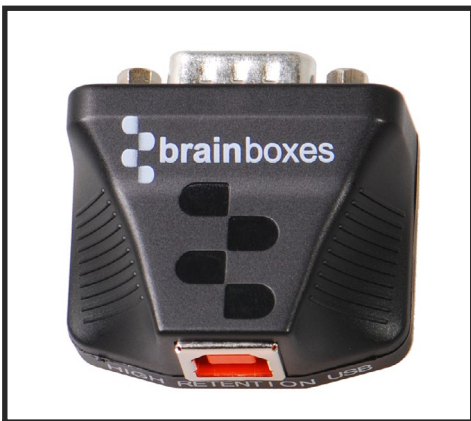
IP-50 rated non-conducting case
