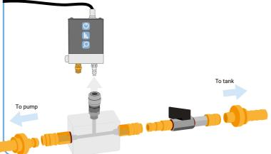
With PicoScope and the WPS500X you can verify the integrity of low-pressure fuel systems. We can look at priming pressure, low pressure associated with priming pumps in tank, fuel filter blockages, leaking pipes hoses or injectors, and aeration within the fuel system. To run this test place the Pico Sight block kit and WPS500X inline on the low pressure side between the high pressure pump and the tank.
