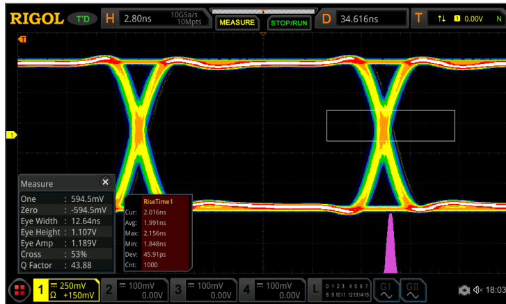
Figure 14: Eye Diagram after debugging and improvements
