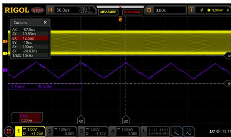
Figure 3: TIE trend graph cursor measurements
