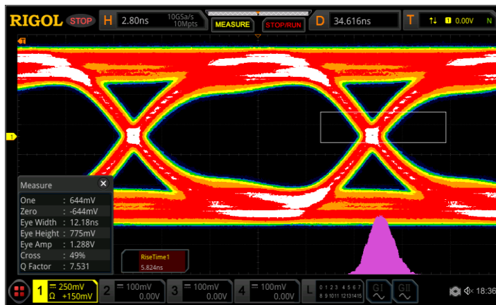
Figure 12: Eye Diagram with improved timing
